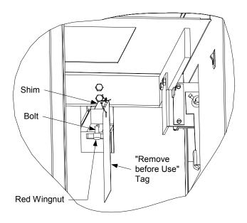
This bolt (with attached red wignut) and shim are used to protect the load cell during shipment. They must be removed before the unit will work properly.
